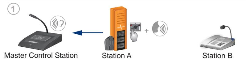
Subscriber at Station A requests the master control station to configure a duplex connection to subscriber at Station B.
