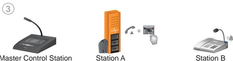
A temporary duplex connection is configured. Operator at Station A lifts his handset and presses his switchboard speak key once briefly. A ringing tone is played back at Station B.
