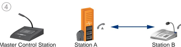
A temporary duplex connection is established as soon as the operator at Station B lifts his handset. Both operators can now speak with each other in duplex mode via handset.
