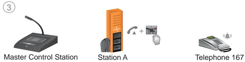
A temporary duplex connection is configured. Operator at Station A lifts his handset and presses the switchboard speak key once briefly. The telephone rings.
