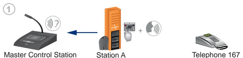
Subscriber at Station A requests the master control station to configure a duplex connection to Telephone 167.
