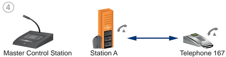
A temporary duplex connection is established as soon as the telephone is picked up. Both operators can now speak with each other in duplex mode.
