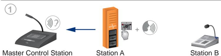
Subscriber at Station A requests the master control station to configure a two-way connection to subscriber at Station B.
