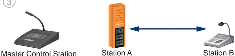
A temporary two-way connection is configured. The subscribers at Station A and B can speak to each other using the corresponding switchboard speak key.
