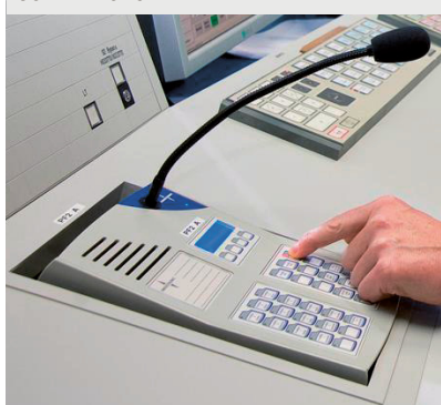
30 DTM 010 installed into a control desk
