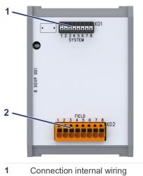
Connection field wiring
