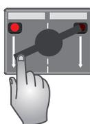
LED is illuminated. The corresponding side of the rocker switch was pressed once previously.
