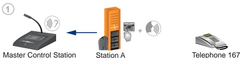
Subscriber at Station A requests the master control station to configure a duplex connection to Telephone 167.
