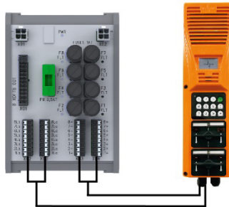
Fig. 6-5: XDFTB connected to intercom station
