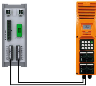
Fig. 6-2: XDTB connected to intercom station
