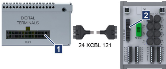
Fig. 6-4: XDG connected to XDFTB
