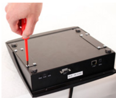
Figure 5-5: Unscrew the cover plate
