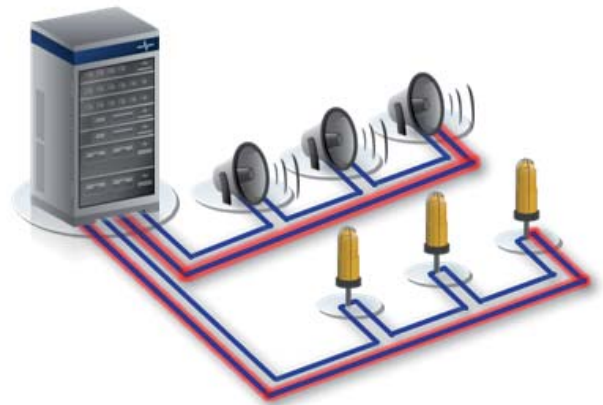
Loop cabling of speakers and beacons
