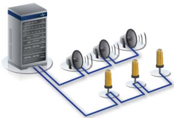
Line cabling of speakers and beacons
